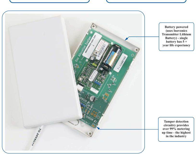
Hydronic baseboards and single speed are metered by measuring run time and water temperature. G.A.S.<sub>TT</sub> is the only system in the industry that has daily tamper detection. The tamper detection mechanism indicates any third party tampering by maintenance staff or residents by detecting cut or disconnected sensor wires and/or malfunctioning zone valves. G.A.S.<sub>TT</sub> uses the industry-standard Inovonics wireless platform for data transmission and collection.
